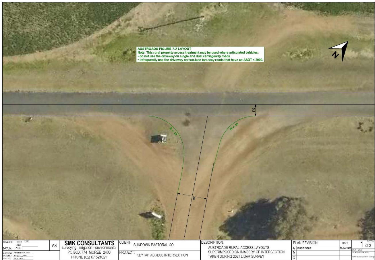
Figure 5: Austroads rural access layout superimposed on 2021 aerial imagery.(also included as Appendix 2)
